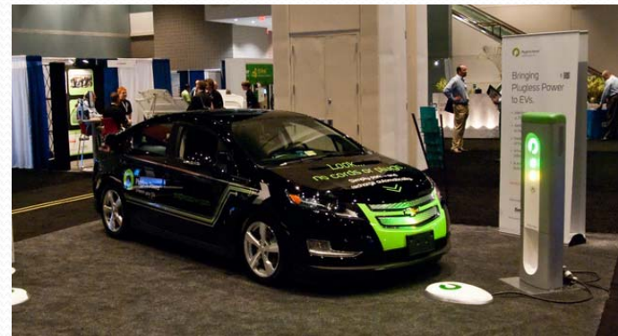
Resonant magnetic coupling charges electrical vehicle.
