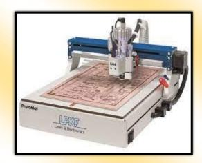
Vacuum table: The integrated vacuum table facilitates processing of flexible materials and securely holds small workpieces down on the working surface.
