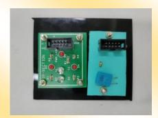
The DHT11 is a basic, low cost digital temperature and humidity sensor. DHT11 is a single wire digital humidity and temperature sensor, which provides humidity and temperature values serially with one-wire protocol. DHT11 sensor provides relative humidity value in percentage (20 to 90% RH) and temperature values in degree Celsius (0 to 50 °C). DHT11 sensor uses resistive humidity measurement component, and NTC temperature measurement component.
