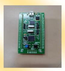
The STM32VLDISCOVERY discovery kit includes an STM32F100 Value line microcontroller in a 64-pin LQFP and an incircuit ST-LINK debugger/programmer to debug discovery applications and other target board applications.
