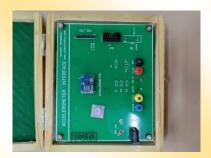
Accelerometer is an electromechanical device that measures the force acceleration due to gravity in g unit. It can be used in applications requiring tilt sensing. The ADXL335 sensor measures acceleration along X, Y and Z axes and gives analog voltage output proportional to the acceleration along these Microcontrollers can process these voltages by converting them to digital signals using ADC.
