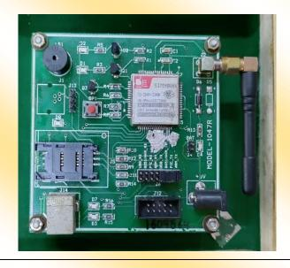
SIM900A Modem can work with any GSM network operator SIM card just like a mobile phone with its own unique phone number. SIM900A GSM/GPRS modem is plug and modem play with RS232 serial communication supported. Hence Advantage of using this modem will be that its RS232 port can be used to communicate develop embedded applications. Applications like SMS Control, data transfer, remote control and logging can be developed. SIM900 modem supports features like voice call, SMS, Data/Fax, GPRS etc.
