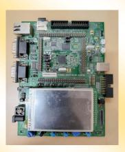
The STM3240G-EVAL evaluation board is a complete demonstration and development platform for the STM32F407IGH6 high-performance 32-bit microcontroller with ARM®Cortex®-M4F processor. The full range of hardware features on the board helps users to evaluate all the peripherals (USB-OTG HS, USB-OTG FS, and Ethernet, motor-control, CAN, microSD ™-card, smartcard, USART, audio-DAC, RS-232, IrDA (up to board MB786 C-07), SRAM, ST-MEMS, EEPROM and others) and to develop applications.
