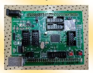
This daughter card consist of 8051-based SST SST89V564RD Microcontroller having following specifications: 25MHz, 3 volt with 32 I/O lines, 3 Timers/Counters, 9 Interrupts/4 priority levels, 64K+8K FLASH, 1K on-chip RAM, SPI, Dual Data Pointers, WDT, 5-channel PCA.
