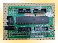
This daughter card consist of high-performance, low-power Microchip 8-bit AVR 8515 RISC-based microcontroller combines 8 KB of programmable Flash memory, 512B SRAM, up to 64 KB external SRAM, and 512B EEPROM. The device supports a throughput of 16 MIPS at 16 MHz and operates between 2.7-5.5 volts.
