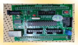
This daughter card is an Arduino Uno board ATmega328P microcontroller and developed by Arduino.cc. The board has 14 digital I/O pins (six capable of PWM output), 6 analog I/O pins, and is programmable with the Arduino IDE via a type B USB cable. It can be powered by the USB cable or by an external 9-volt battery, though it accepts voltages between 7 and 20 volts.
