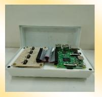
a 64-bit quad core processor running at 1.4GHz, dual-band 2.4GHz and 5GHz wireless LAN, Bluetooth 4.2/BLE, faster Ethernet, and PoE capability via a separate PoE HAT. The board has following specifications:
