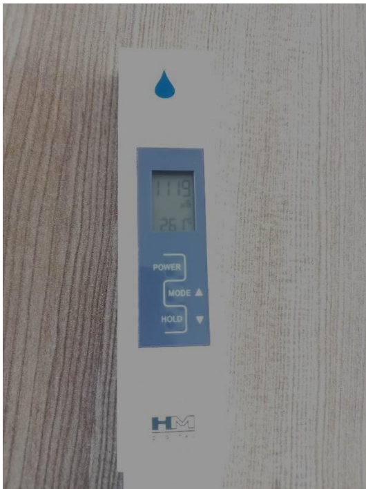
Photograph 6: The testing of water quality of the water sample collected from the village Bishanpura, using AP-2: AquaPro Water Quality Tester
