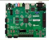
ZedBoard<sup>™</sup> is a low-cost development board for the Xilinx Zynq®-7000 SoC. This board contains everything necessary to create a Linux, Android, Windows® or other OS/RTOS-based design. Additionally, several expansion connectors expose the processing system and programmable logic I/Os for easy user access. Take advantage of the Zynq-7000 SoC's tightly coupled ARM® processing system and 7 series programmable logic to create unique and powerful designs with the ZedBoard.
