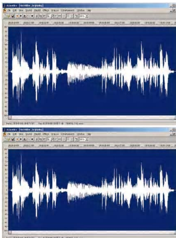
Fig. 3: The signal level comparisons between a WAV carrier file before (above) and after (below) the LSB coding is done
