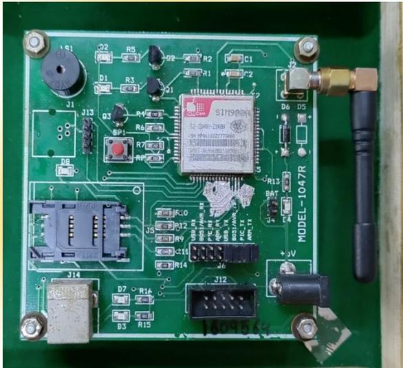
SIM900A Modem can work with any GSM network operator SIM card just like a mobile phone with its own unique phone number. SIM900A GSM/GPRS modem is plug and play modem with RS232 serial communication supported. Hence Advantage of using this modem will be that its RS232 port can be used to communicate and develop embedded applications. Applications like SMS Control, data transfer, remote control and logging can be developed. SIM900 modem supports features like voice call, SMS, Data/Fax, GPRS etc.
