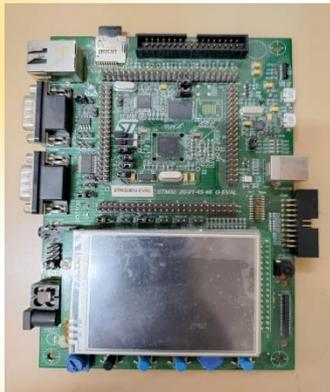
The STM3240G-EVAL evaluation board is a complete demonstration and development platform for the STM32F407IGH6 high-performance 32-bit microcontroller with ARM®Cortex®-M4F processor. The full range of hardware features on the board helps users to evaluate all the peripherals (USB-OTG HS, USB-OTG FS, and Ethernet, motor-control, CAN, microSD™-card, smartcard, USART, audio-DAC, RS-232, IrDA (up to board MB786 C-07), SRAM, ST-MEMS, EEPROM and others) and to develop applications.
