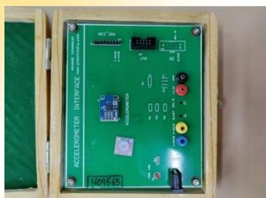
Accelerometer is an electromechanical device that measures the force of acceleration due to gravity in g unit. It can be used in applications requiring tilt sensing. The ADXL335 sensor measures acceleration along X, Y and Z axes and gives analog voltage output proportional to the acceleration along these 3 axes. Microcontrollers can process these voltages by converting them to digital signals using ADC.
