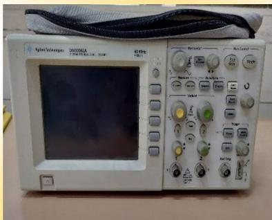
A digital storage oscilloscope (DSO) is an oscilloscope which stores and analyses the input signal digitally rather than using analog techniques. It is now the most common type of oscilloscope in use because of the advanced trigger, storage, display and measurement features which it typically provides.
