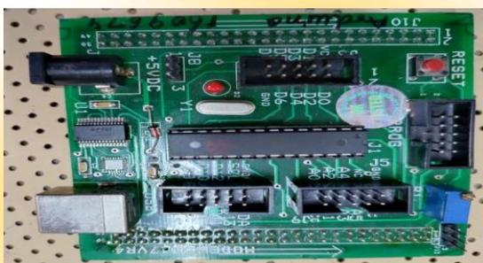
This daughter card is an Arduino Uno board ATmega328P microcontroller and developed by Arduino.cc. The board has 14 digital I/O pins (six capable of PWM output), 6 analog I/O pins, and is programmable with the Arduino IDE via a type B USB cable. It can be powered by the USB cable or by an external 9-volt battery, though it accepts voltages between 7 and 20 volts.
