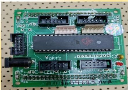
This daughter card consist of high-performance, low-power Microchip 8-bit AVR 8515 RISC-based microcontroller combines 8 KB of programmable Flash memory, 512B SRAM, up to 64 KB external SRAM, and 512B EEPROM. The device supports a throughput of 16 MIPS at 16 MHz and operates between 2.7-5.5 volts.
